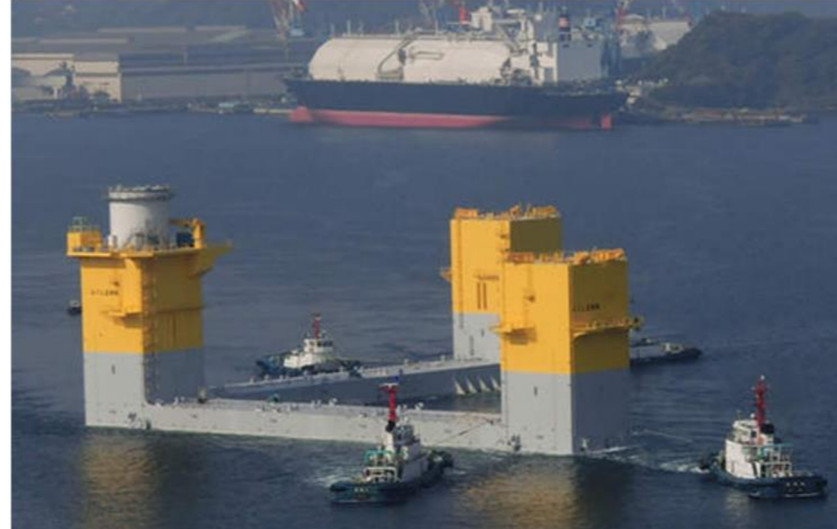
A 7MW oil pressure drive-type floating wind turbine will be installed on three-column semi-sub floater. Credit: Fukushima Offshore Wind Consortium.
